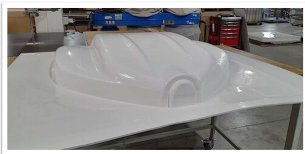
Thermoformage capot Baker-Prax
