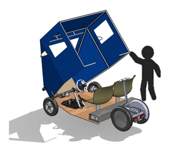
• A jack at the back of the vehicle allows one to remove the segway when parked.
