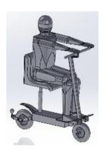
• This "roue jocket" is present at the back of the vehicle to prevent scale of the vehicle during travel also.
